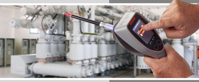
Once a leak has been localised, the push of a button puts the instrument into "Measuring Mode" if desired. In this mode the handgun display is switched to numerical reading. It is now possible to precisely measure the leak, with the leak rate displayed on the handgun screen.
